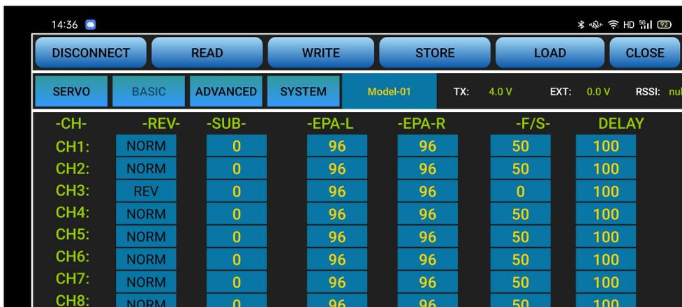
**REV:** Defines the relationship between the transmitter controls and the receiver output for channels with options of NORM and REV. Make sure to check all servos move to the correct direction as wish under control. Make sure to check all servos move to the correct direction under control.
