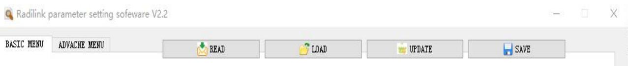
**READ:** T8S data will be read and displayed on computer when click “READ”. The two LEDs at the rightmost will flash once at the same time with two D sounds .
