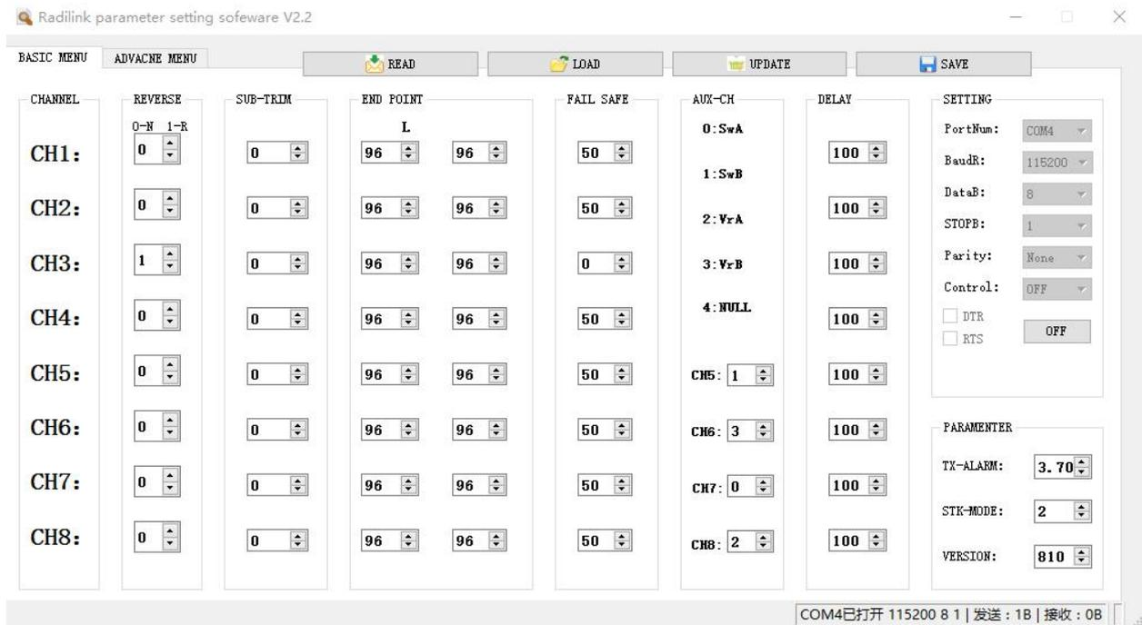
**REVERSE:** Defines the relationship between the transmitter controls and the receiver output for channels with option of NORM and REV. Refer to 3.3.2-REV (P7) for more details.
