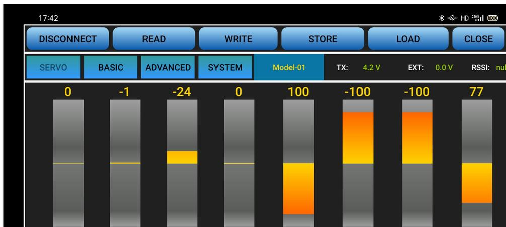
**(DIS)CONNECT:** When APP is opened on the mobile and T8S is powered on, click CONNECT and a list of Bluetooth devices will pop out and select the RadioLink device to make connection. The two leds at the rightmost will flash in turn with DD sounds, **press any of the trimmer buttons to stop the DD sounds** and the servo range will display on the APP. If fails, press DISCONNECT and CONNECT again.
